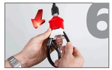
After clicking-in the metal end of the chicken loop under the stainless steel lever mechanism, let go of the red plastic part in your left hand to close the system. Now the quick release safety system is ready to be used
