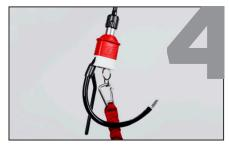
Now the chicken loop is open. This rapidly kills all the power of the kite. You are now connected to the kite only via the safety leash, which should also be releasable in a case of extreme emergency.
