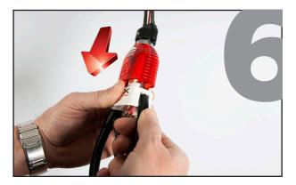
After clicking-in the metal end of the chicken loop under the stainless steel lever mechanism, let go of the red plastic part in your left hand to close the system. Now the quick release safety system is ready to use again.
