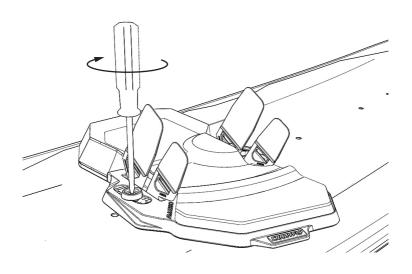
**7.** Fully tighten the screws. Please check the footpad screws after the first few rides, as they may come loose. If loose, make sure to fully tighten the screws.
