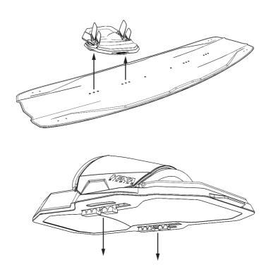
**15.** If further adjustments for the footstrap position and footpad position are needed, undo the screws completely. Lift up the Hexa Binding, push the Quttro Stix down so they pop out of the Fusion Frame. Adjust the Quattro Stix to the desired position and pop them back in the Fusion Frame. Mount the Hexa Binding back on the board to the desired position and fully tighten your screws.
