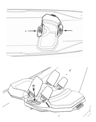
**5.** Put 2 pcs Hexa washers in place, one to the left and the other one to the right side of the Hexa footpad. Make sure the holes in the washer are aligned with the inserts on the board. Tighten 2 pcs screws slightly - left and right side of the Hexa footpad.
