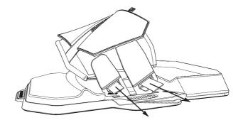
**8.** Take the Hexa footstrap Right and open the velcro. Thread the velcro through the Quattro Stix. It is best to start on the Quattro Stix Long in the left side of the Hexa footpad right (inside of the foot). Then continue with threading the velcro through the Quattro Stix Short on the same side.
