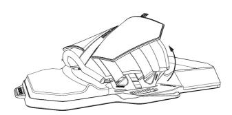
**9.** Slide the Quattro Stix inside the footstrap. Slightly tighten and close the threaded velcros. Leave the velcros a bit loose and close the top velcro. Leaving the velcro loose will make threading the velcro on the other side of the footpad easier.
